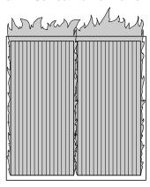
Figure 22 - Incorrect Burner Flame Pattern
